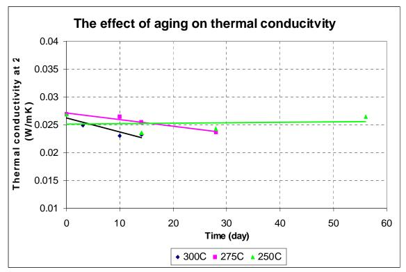
Figure 6 Thermal conductivity at 200°C after highly accelerated thermal aging
