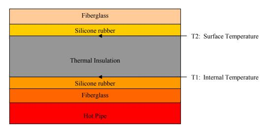
Figure 4 Specimen structure for the surface temperature test
