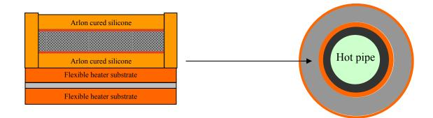
Figure 9 Arlon Flexible Heater Substrates Insulate with Arlon Insulation
