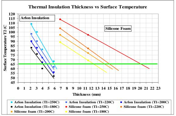
Figure 5 The effect of thickness on outside surface temperature for different thermal insulation materials
