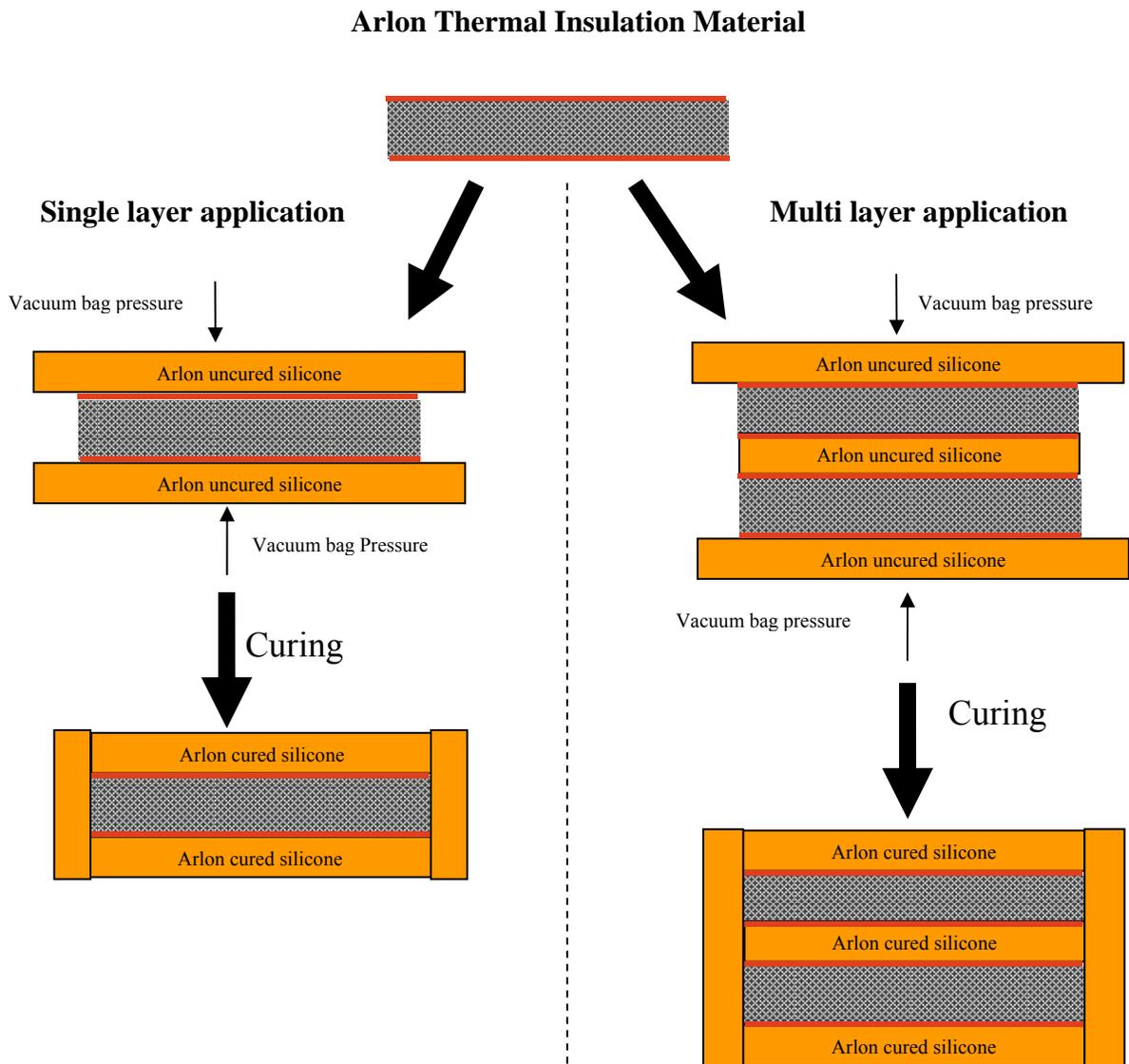
**Figure 8 Vacuum bag curing to seal the edges for particle free applications**
