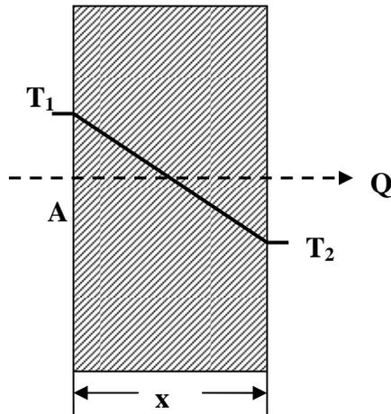
**Figure 2 Schematic of thermal conduction**
