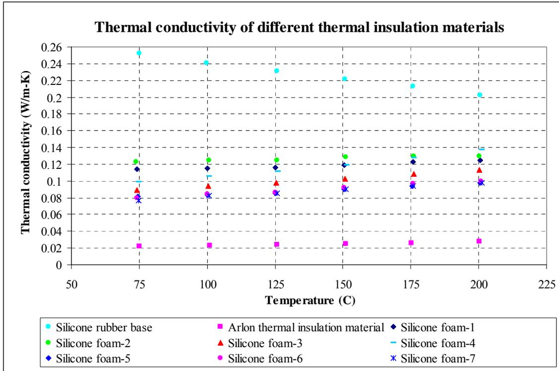
**Figure 3 Thermal conductivity of different thermal insulation materials**
