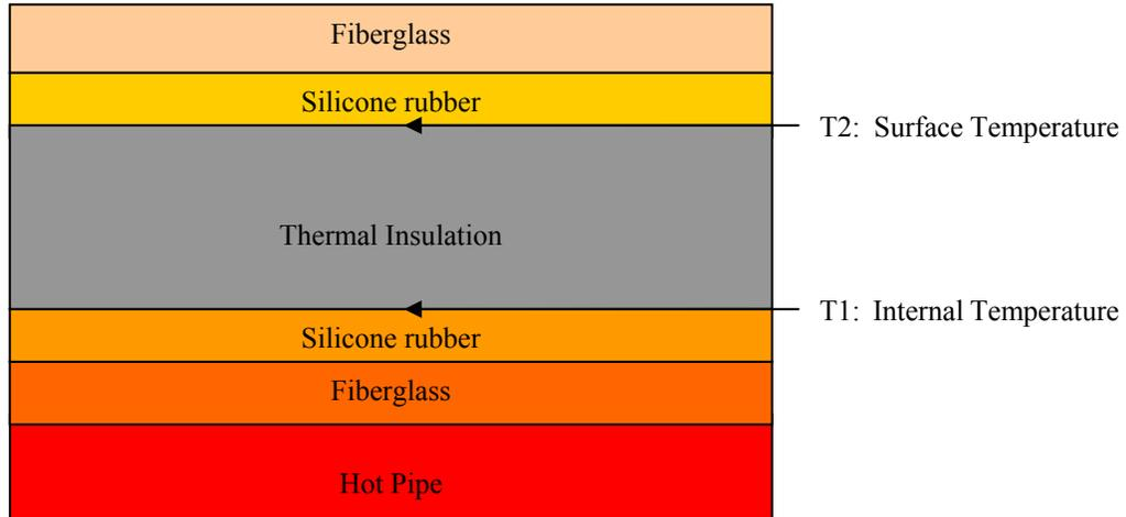
Figure 4 Specimen structure for the surface temperature test
