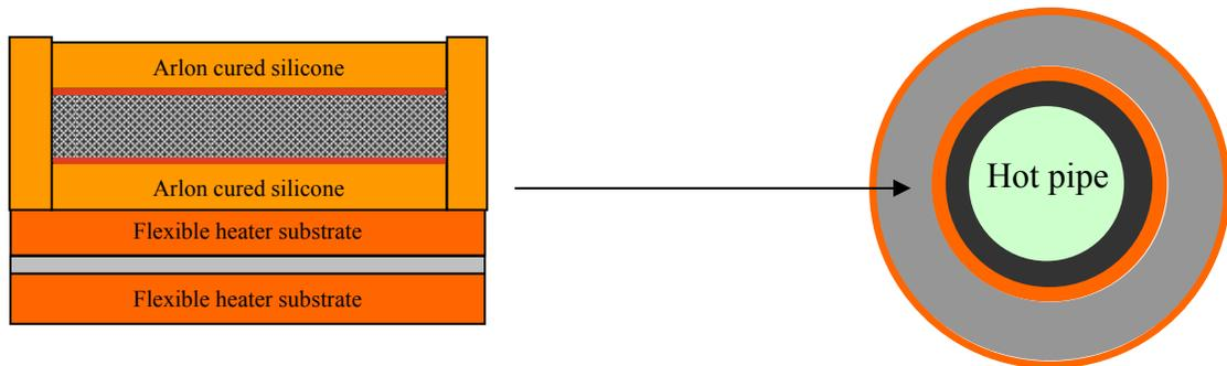
**Figure 9 Arlon Flexible Heater Substrates Insulate with Arlon Insulation**
