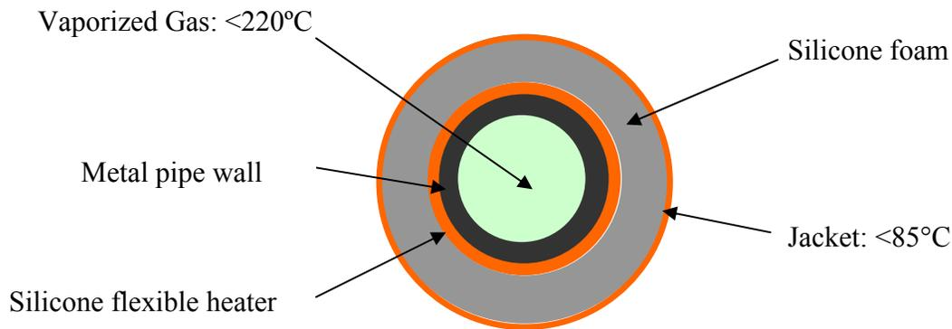
**Figure 1 Heating assembly for gas pipe in the semiconductor industry**
